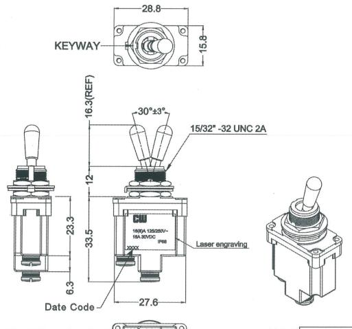
Rating: 16(8)A 125/250V~ T55 Electrical Life: 10,000 cycles Mechanical Life: 50,000 cycles
