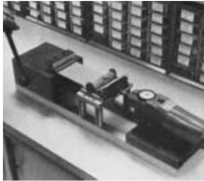
Test to determine the force for cover pull-off from base of connector
